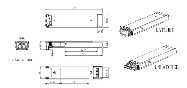
XFP Transceiver (dimensions are in mm)
