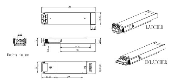
XFP Transceiver (dimensions are in mm)
